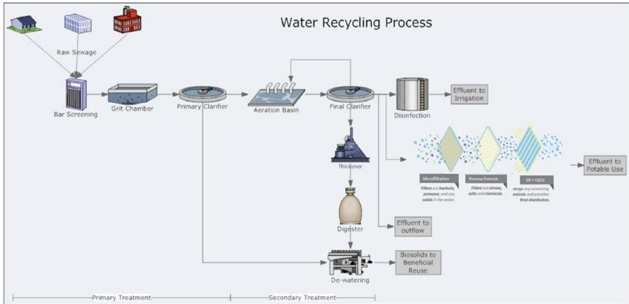
Primary sedimentation follows, eliminating most of the suspended materials and, if some of these solids are biodegradable, the biochemical oxygen demand (BOD) is typically reduced. Then, secondary treatment usually involves a biological process. Microorganisms in suspension (in the “activated sludge” process), are used to remove biodegradable organic material.
